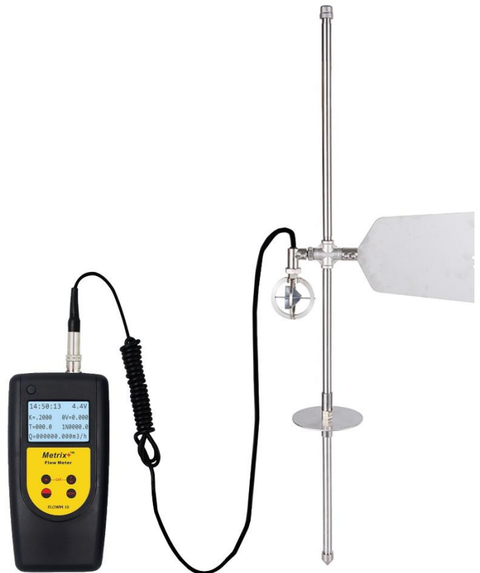
FLOWM 10 (upto 10m/s) has about 1.8m long sensor with 6 extension rods
